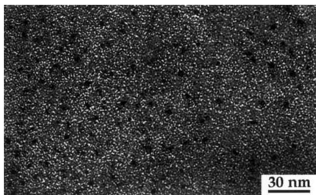
Fig. 1 TEM micrograph of PS-g-PAA micelles stained with Pb(Ac)_3 and cast from toluene
